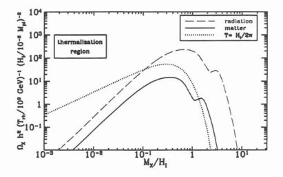
FIGURE 2. The contribution of gravitationally produced WIMPZILLAS to  $\Omega_X h^2$  as a function of  $M_X/H_I$ . The shaded area is where thermalization may occur if the annihilation cross section is its maximum value. Also shown is the contribution assuming that the WIMPZILLA is present at the end of inflation with a temperature  $T = H_I/2\pi$ .
