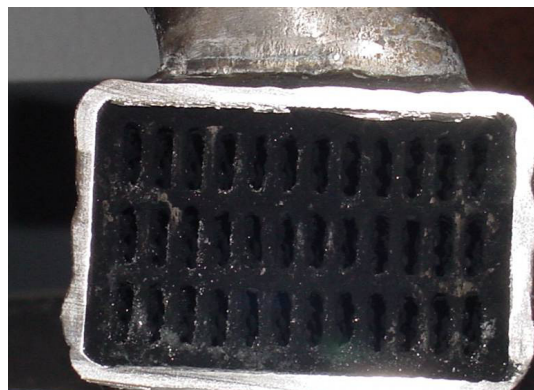
Figure 1.1 – Deposits at EGR cooler inlet following 200 hour engine fouling test [2]
