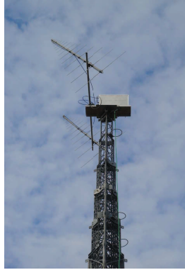
Figure 5.3: A typical setup for sky calibration. To minimize the capture of unwanted signals the antennas are pointing at 45^\circ above horizontal.
