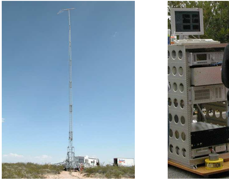
Figure 5.1: MOSS Radar picture. The system was a monostatic radar which used a large dual polarization log periodic antenna, balanced by a set of lead counterweights. The ground electronics consisted of (from the top) a signal generator, RF ground box, a computer housing a PCI digitizer, a radar power supply and an AC power backup unit
