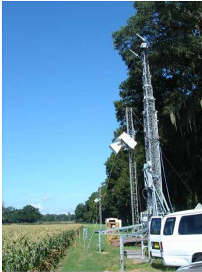
Figure 5.2: A photo of the Bistatic Radar. Antennas are separated by a 6' custom made steel beam. The height of the tower is varried between 12m and 35m. The incidence angle is set manually for every antenna. In this picture the antennas are pointing up for calibration purposes.
