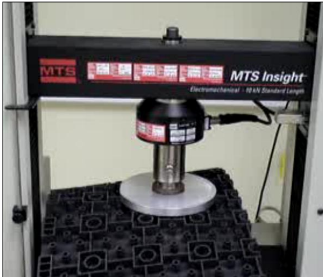
Figure A.1: MTS material testing machine compressing a mat in a laboratory test
