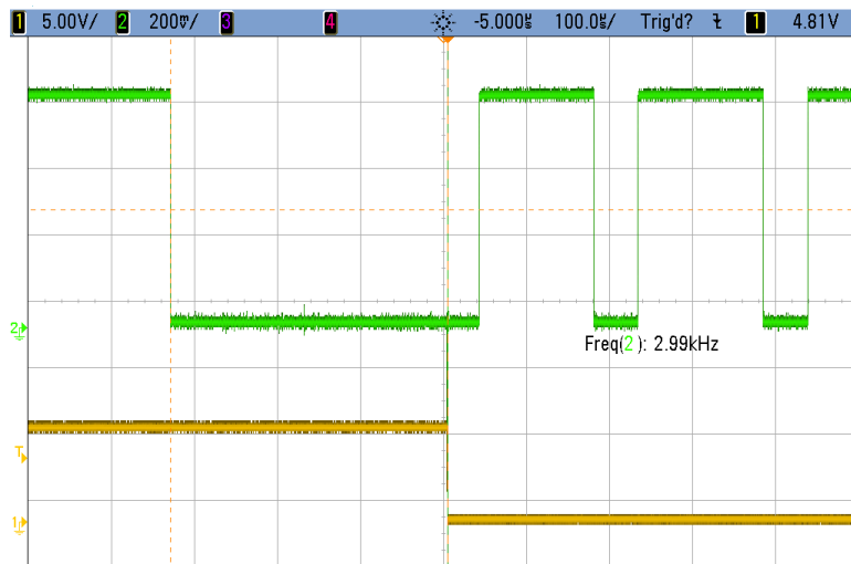
Figure 5.24. Ring oscillator switching between two different capacitive loads, from a larger capacitance (State 2) to a smaller capacitance (State 1), after optical triggering.
