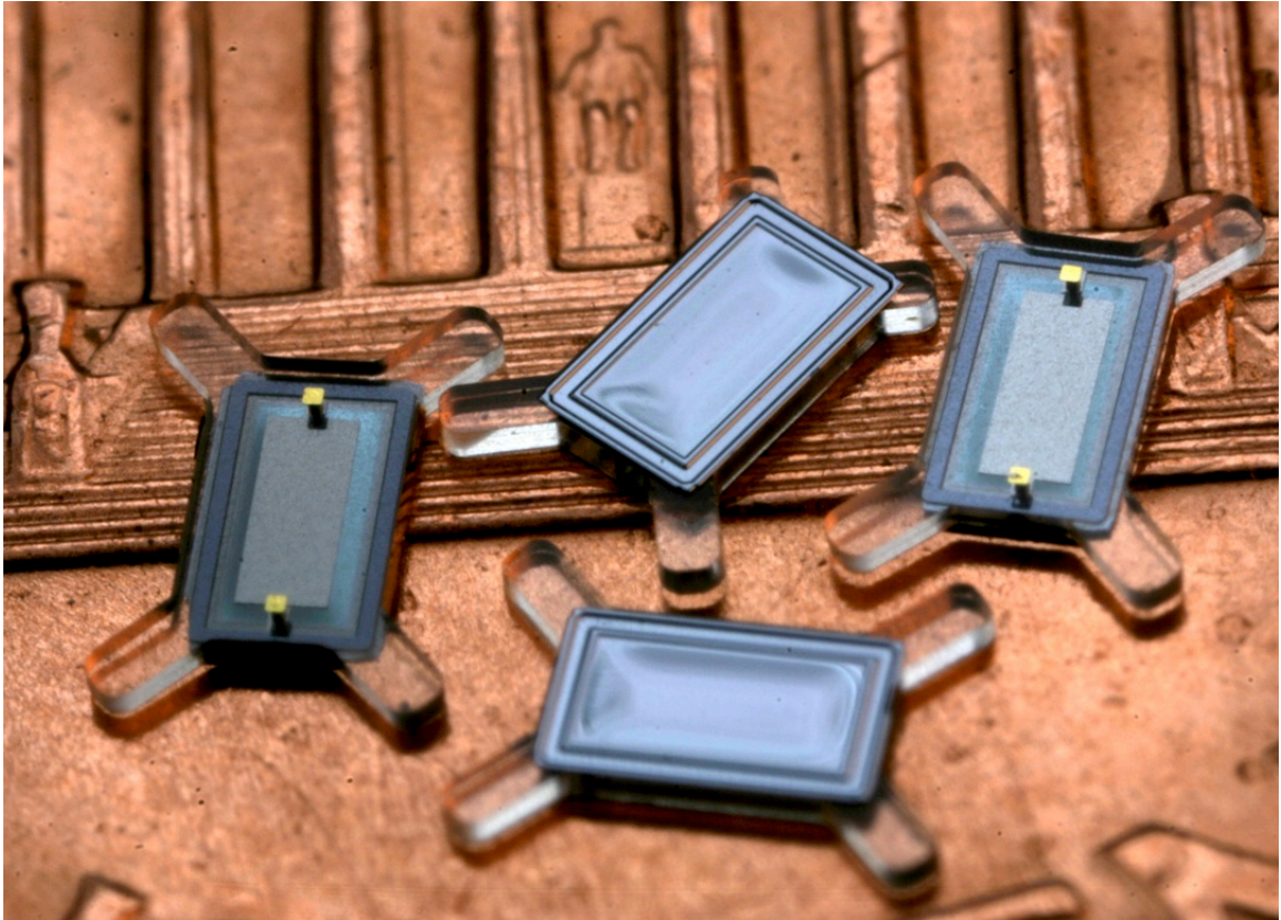
Figure 3.17. Four pressure sensors fabricated with the silicon-in-glass process. Two sensors in the center show the deflected diaphragm and two sensors on the left and right show the backside of the sensor.
