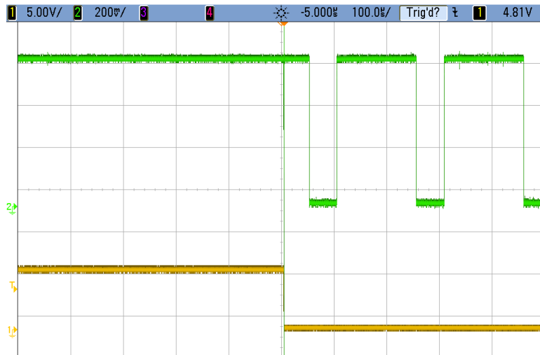
Figure 5.22. Ring oscillator startup (top), entering State 1 after optical trigger (bottom).
