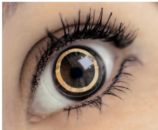
Figure 1.3. The SENSIMED Triggerfish uses a contact lens to measure intraocular pressure [22]. The external power patch is not shown.
