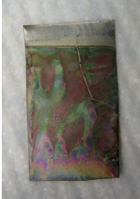
Figure 3.2: Macroscopic image of a titania nanotube array created from titanium foil. The top portion is the un-anodized titanium and the multicolored area is composed of titania nanotubes.
