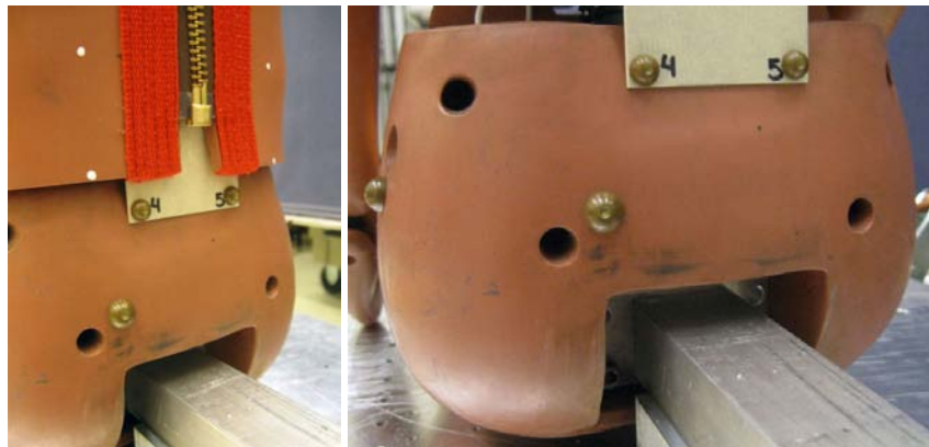
Figure A4. Pelvis in fixed position and sphere targets on pelvis and spine box
