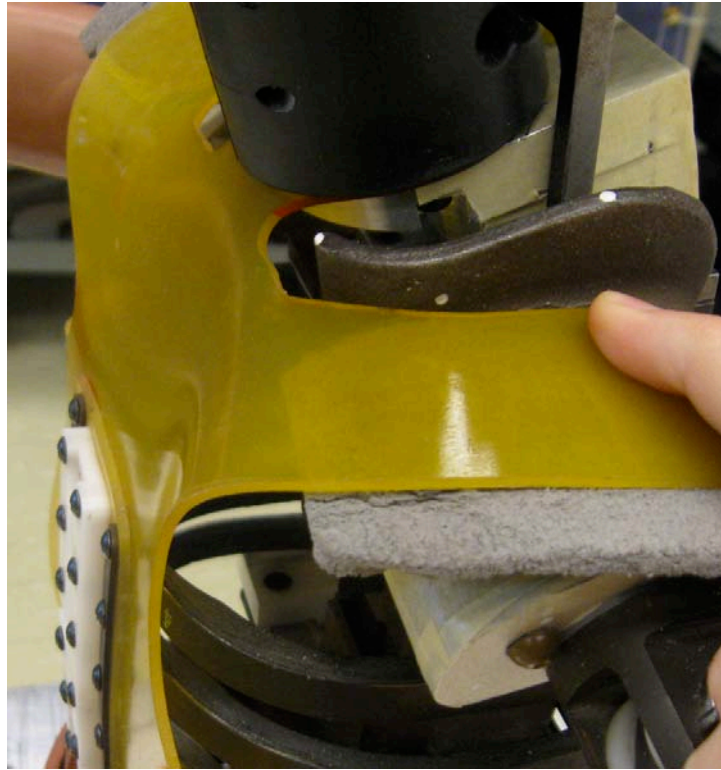
Figure 16. Bib assembly fit on ATD shoulder with clavicle link rotated down and clavicle rotated rearward.
