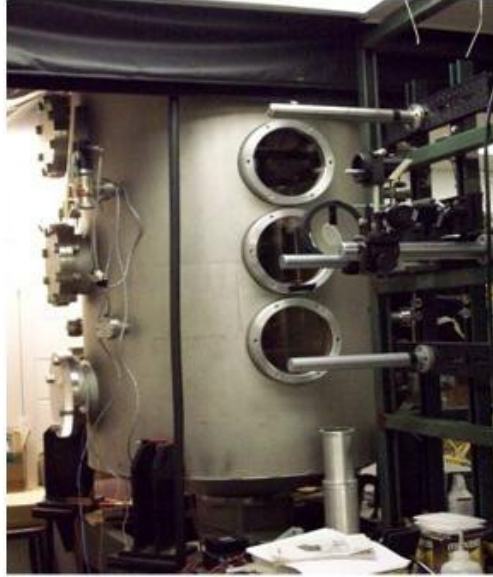
Figure 5: Vacuum vessel containing underexpanded-jet freestream flowfield.
