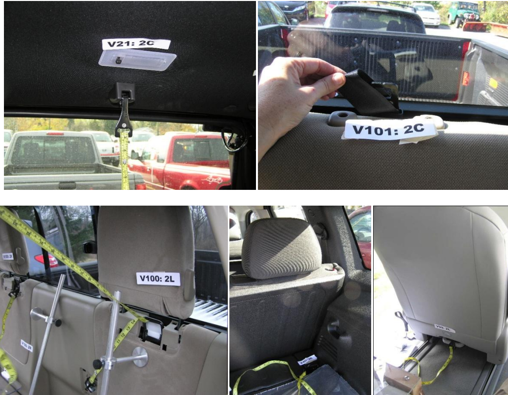
Figure 28. Tether locations on the roof, back wall, 2 nd row, floor, and under seat.
