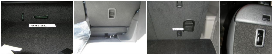
Figure 31. Confusing tether hardware in the BMW Minicooper, Honda Pilot, Honda CRV, and Porsche Cayenne.
