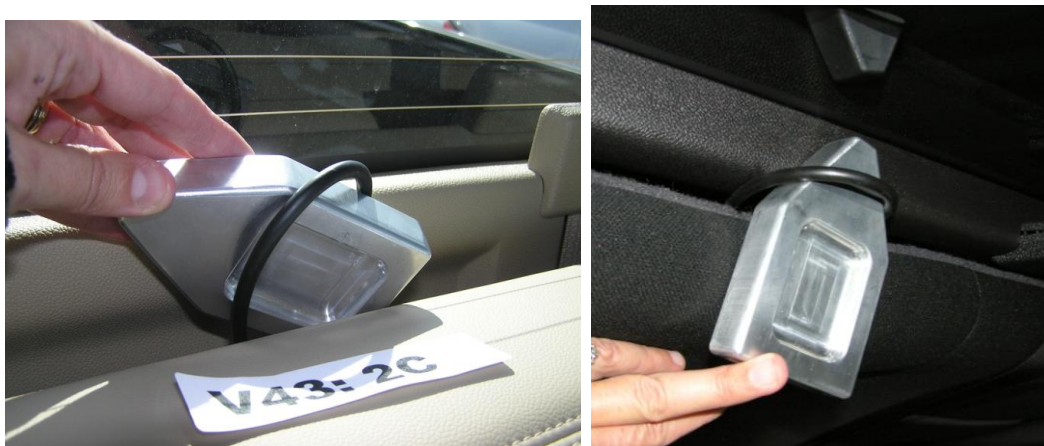
Figure 63. Using the tether router clearance tool (left=pass, right=fail).
