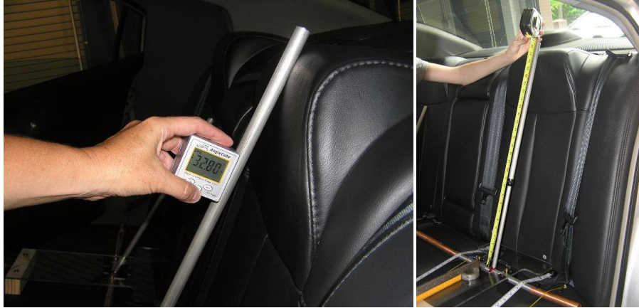
Figure 10. Measuring the angle and distance to the tangent of the head restraint.
