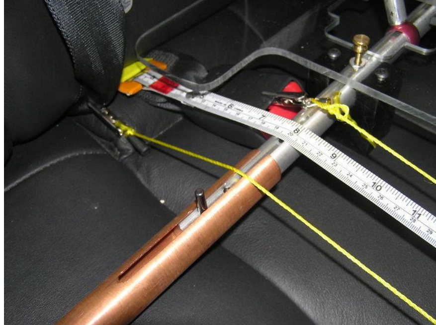
Figure 5. Documenting location of lower anchors and lateral locations of belt hardware. The hooks used to attach the measuring tape to the lower anchors were also marked with colored electrical tape as shown in Figure 6. The width of the tape is 2 cm, so the depth of the anchors within the bight can be estimated by what color is visible. The center photo of Figure 6 illustrates an anchor with less than 2 cm of depth because the blue tape is visible, while the right photo in the figure depicts an anchor with 4-6 cm of depth because the yellow tape is visible.
