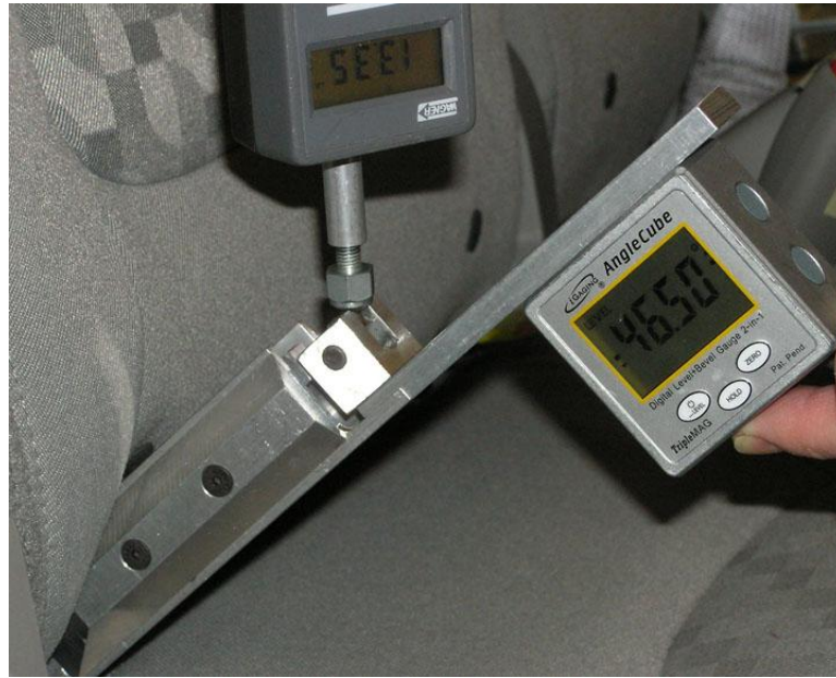
Figure 56. Method of measuring lower anchor clearance.
