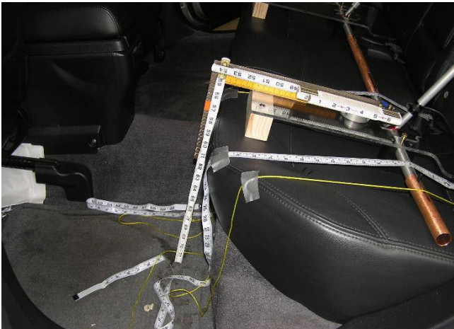
Figure 14. Measuring floor height.
