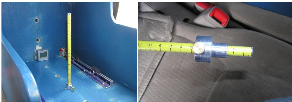
Figure 11. Measuring seat profile relative to surface of child restraint fixture.
