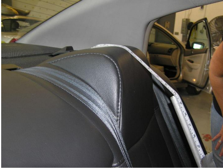
Figure 8. Measuring the wrap distance from tether anchor to the estimated R-point.
