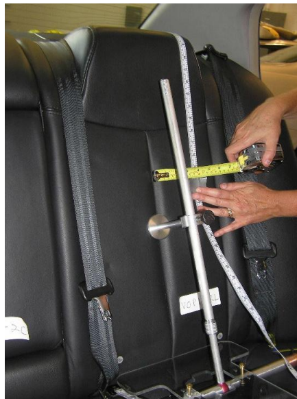
Figure 9. Measuring lateral distance from tether anchor to vehicle seat centerline.
