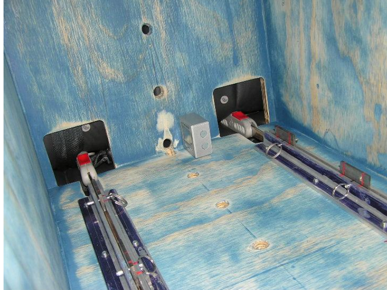
Figure 58. Measuring pitch angle of fixture when installed at a LATCH position.
