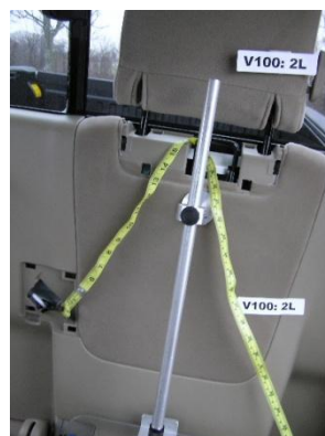
Figure 33. Toyota Tacoma tether anchor configuration for 2L position. The yellow tape traces the intended tether path.
