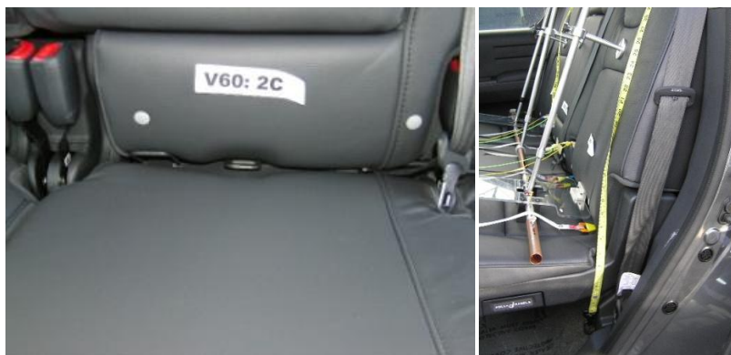
Figure 32. Honda Ridgeline tether anchor locations for center seating position (left) and outboard seating positions (right, yellow tape indicating path of tether to anchor).
