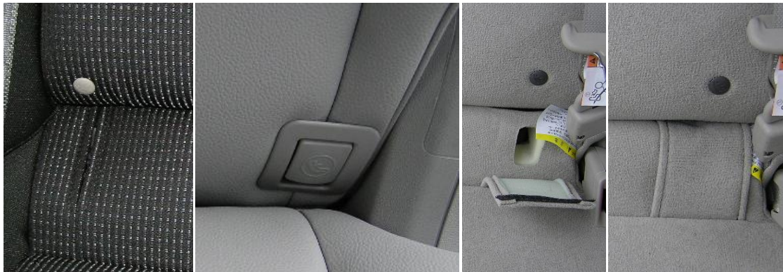
Figure 26. Types of lower anchor coverings: slit, door, flap (open and shut).
