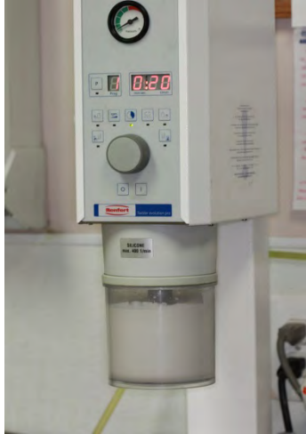
Figure 15. Twister Evolution Pro, vacuum mixing unit, Renfert II, USA
