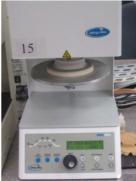
Figure 24. Whipmix Pro 100 ceramic oven, USA.
