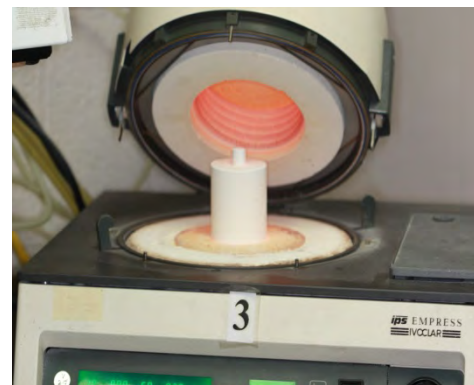
Figure 20. Investment cylinder set-up with a pressable ceramic disposable plunger system, Vacalon, OH, USA.
