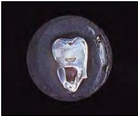
Figure 1. Sectioned experimental specimen mounted in Koldmount acrylic.
