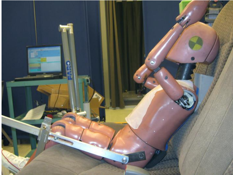
Figure 6. Fixture used to measure distance from hips to front of seat cushion. A foam wedge is used to prevent contact between the head and seat. (See Appendix 1).
