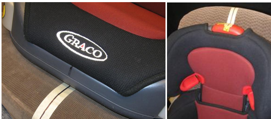
Figure 19. Aligning center planes of booster and vehicle seat
