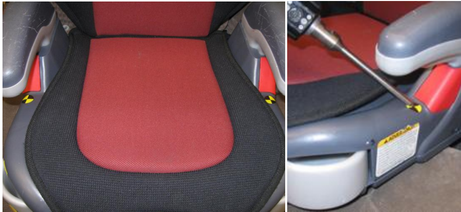
Figure 17. Example bilaterally symmetrical points on booster seat
