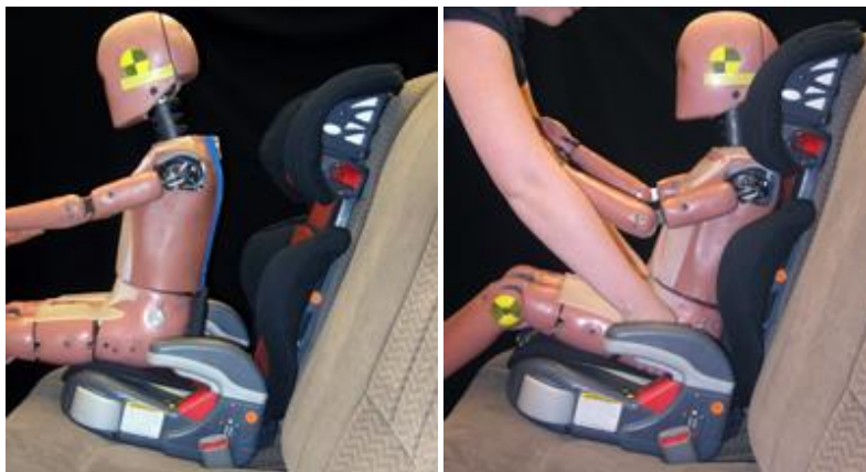
Figure 22. Moving the ATD rearward in the seat
