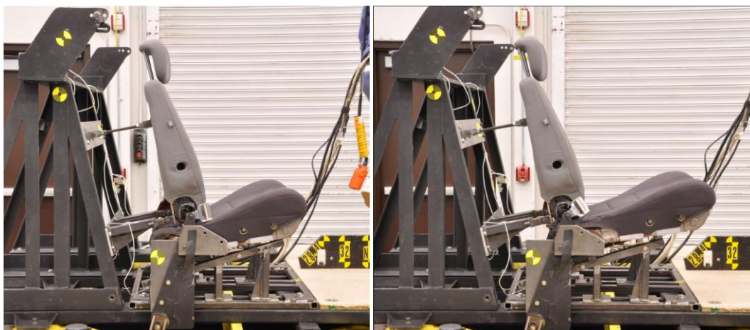
Figure 1. Side view of vehicle seat configured to cushion lengths of 350 (left) and 450 mm (right).
