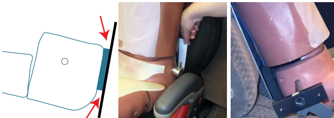
Figure 23. Six-year-old ATD pelvis-positioning pad parallel and in minimal contact
