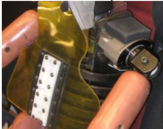
Figure 16. Example of 1/2 inch thick shoulder spacer
