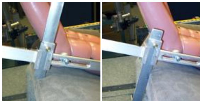
Figure 29. Moving the slider forward until the arm drops.
