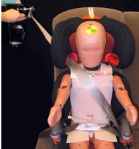
Figure 41. Feeding the shoulder belt into the retractor
