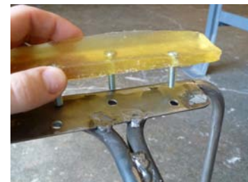
Fig. 13 - Cast urethane mounts get laminated to the chairs and fastened to the frame with a nut
