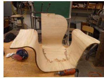
Fig. 15 - The last layup which included armrests, half of the form has been cut out
