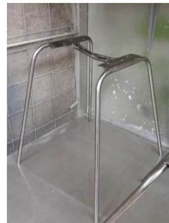
Fig. 17 - Steel rod base after sanding and steel wool
