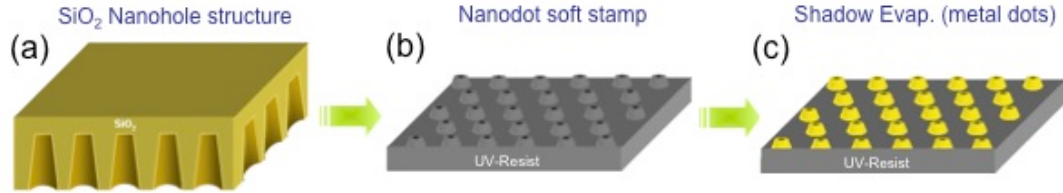
Figure 6.1 Schematic of the process for fabricating plasmonic nanostructures: (a) SiO 2 nanohole type structure; (b) Nanodot soft stamp; (c) Plasmonic metal nanodots.
