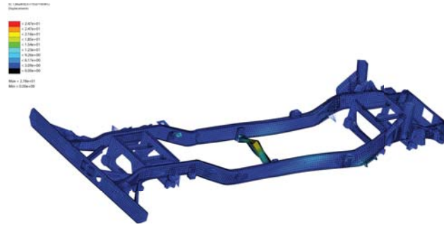
Figure 5.5: The 30 th mode shape of the healthy high mobility multipurpose wheeled vehicle (HMMWV) frame
