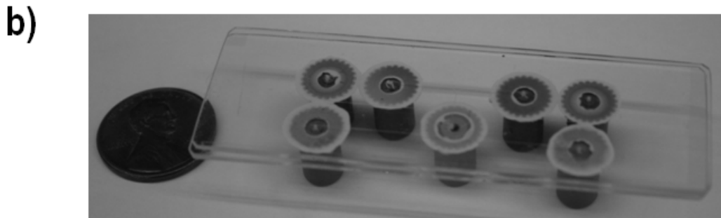
Figure 2.2. Scheme of Islet perfusion glass microchip (a) with 80 \mu\text{m} deep and 120 \mu\text{m} half width channels: droplets are formed at the interface of the aqueous (black) and oil (grey) phases and transported through hydrophobically modified channels and capillary to a laser induced fluorescence photodetection system. All flow was driven by external syringe pumps as depicted. An image of the device inverted to display channels with a cent piece for reference (b) and a cartoon of the FPIA for low and high insulin concentrations (c) are shown.
