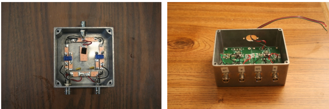
Fig. 5.3: Picture of the detector system (a) and two preamplifier circuits (b).
