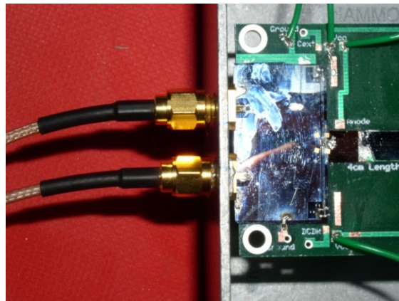
Fig. 5.32: The assembly of the planar detector with the TIA.
