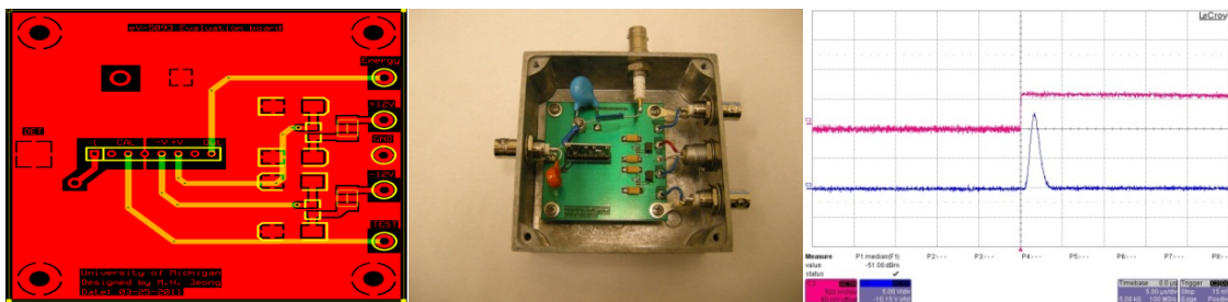
Fig. 5.51: The PCB layout for the eV-5903 preamplifier (left), its picture (middle) and acquired signal (right, pink) and shaped signal (right, blue).
