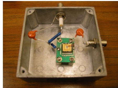
Fig. 3.91: Planar type CZT detector with multiple guard-rings.
