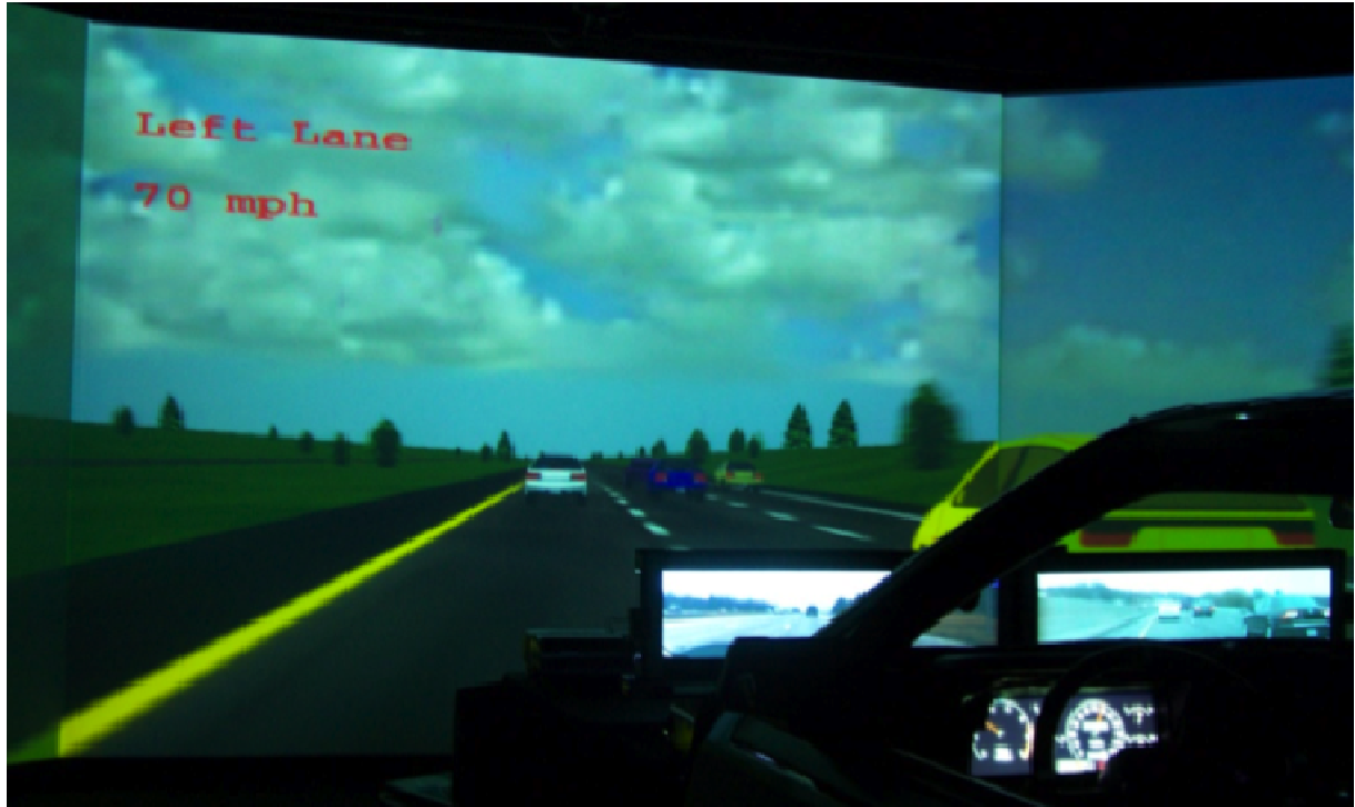
Figure 5. Anchor Projection Screens on the Hood
