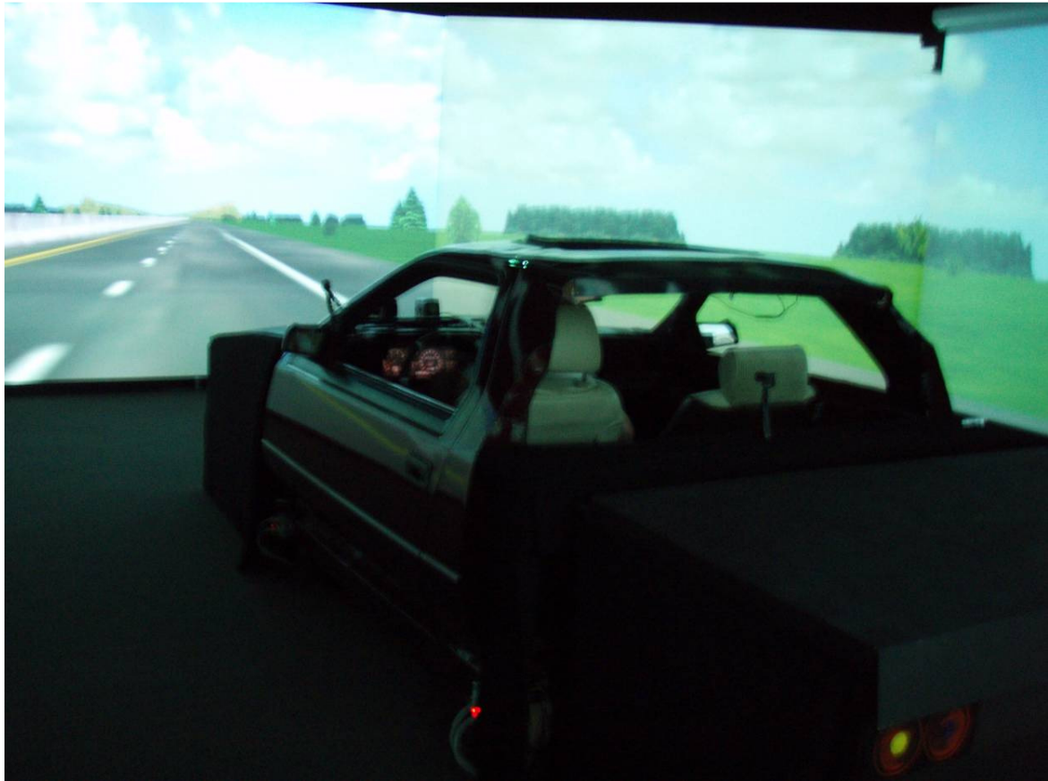
Figure 8. Simulator cab, front screen, front-right screen, and front-side screen
