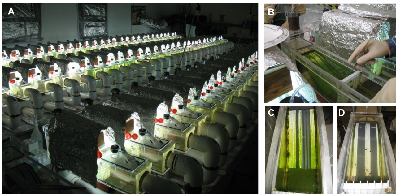
Fig. 1. Experimental flumes used in the present study. (A) We manipulated the presence or absence of three types of common stream algae in a set of 81 recirculating laboratory flumes and then exposed the developing biofilms to three initial concentrations of titanium dioxide (TiO 2 ) nanoparticles (0, 0.1, or 1.0 ppm). (B) Over the course of 32 d, or approximately 10 generations of cell division, we sampled biofilms from “tape-strips” that were placed on the polyvinyl chloride growth surfaces in each flume. This allowed us to collect time series of biofilm biomass without destructive sampling. (C, D) After 32 d of growth, 23 individual Physa acuta , a common freshwater snail, were added to flumes and allowed to feed for 72 h. C and D give one example of algal biomass before and after snail addition.
