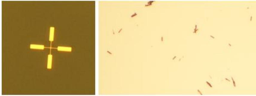
Figure 6.7 (left) Alignment marks used to identify exact position of a single nanowire dispersed on top of \text{SiO}_2 . The minimum feature size is 1\mu\text{m} . (right) Optical micrograph of dispersed nanowires.
