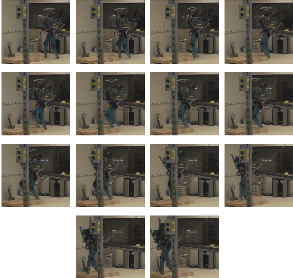
Figure G.1: Snapshot: experiment of step-up of 12.5 cm platform. Snapshots are at an interval of 100 msec. The snapshots progress temporally from left to right and from top to bottom.
