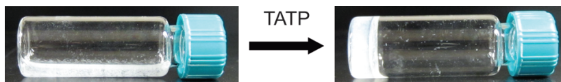
Figure 5.1. A gel forms within 30 min of adding TATP (2.5 mg) to a vial containing thiol 1 (36 mM) and TsOH (1.3 M) in MeOH.
