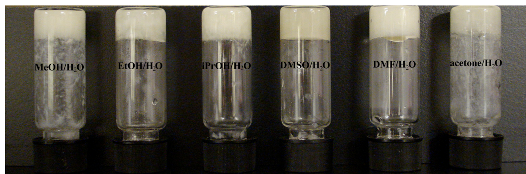
Figure S5. Gel of 2 (26 mM, formed by heat/cool-induced gelation) in a series of organic solvent/water mixtures.
