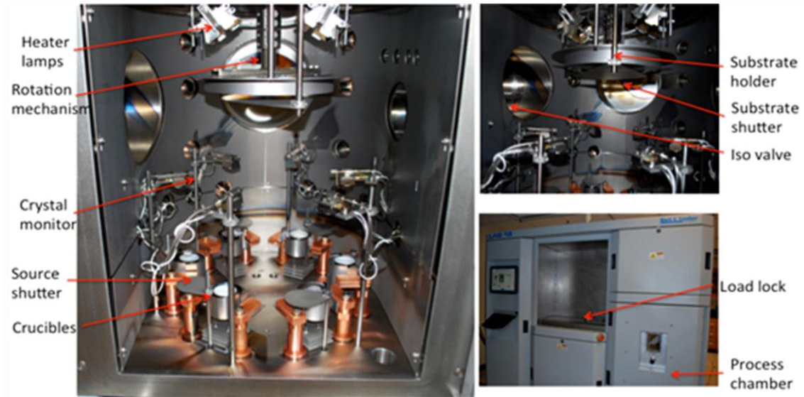
Figure 3.2 Co-evaporation system for (Bi,Sb)Te-based thin films. Basic parts inside the deposition chamber and the exterior of the tool are shown.
