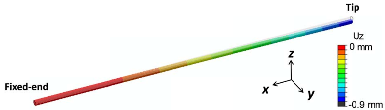
Figure 4.10. FEA model for needle deflection model at 30 mm needle insertion depth, with the overlaid un-deformed needle. Needle deflection (in m) occurred in the z -direction.
