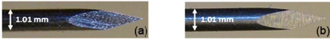
Figure 3.2. Trocars made of (a) AISI 304 stainless steel and (b) tungsten carbide in 6% cobalt.
