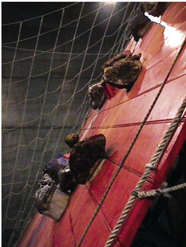
Figure 17. Airbag test platform dipping at 60^\circ in vacuum chamber with rocks attached. Slats that make up platform are \sim 30 cm wide. Net in background is to constrain bounces of airbag clad lander. Rocks are sharp andesites attached to platform, some with concrete bases. Rocks are covered with chalk to record which rocks produced tears or other failure of the bags.
