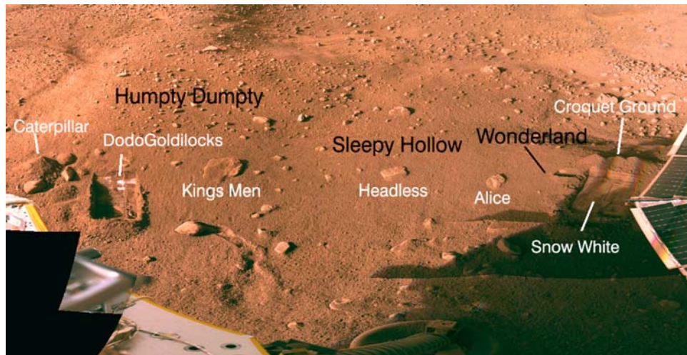
Figure 3. Color view of terrain to the north of the Phoenix Lander acquired relatively early in the mission and showing selected RA excavations, including the trenches Dodo-Goldilocks and Snow White, together with the dump piles Caterpillar and Croquet Ground. Trenches were excavated on the side of the Humpty Dumpty polygon, on top of the Wonderland polygon, in the trough inboard from Humpty Dumpty, and in the gentle swale between these two polygons (Sleepy Hollow). During the mission the RA mistakenly moved the rock Alice and on purpose moved Headless and King’s Men. Note the rock inboard from King’s Men that apparently moved by sliding as thruster exhaust impinged onto the surface during landing. Pits and scour zones can be seen in full resolution versions of the mosaic that extend beyond the RA work volume. For reference the Dodo-Goldilocks trench is ~22 cm wide. Frames obtained from SSI mission success panorama (completed on sol 53).
