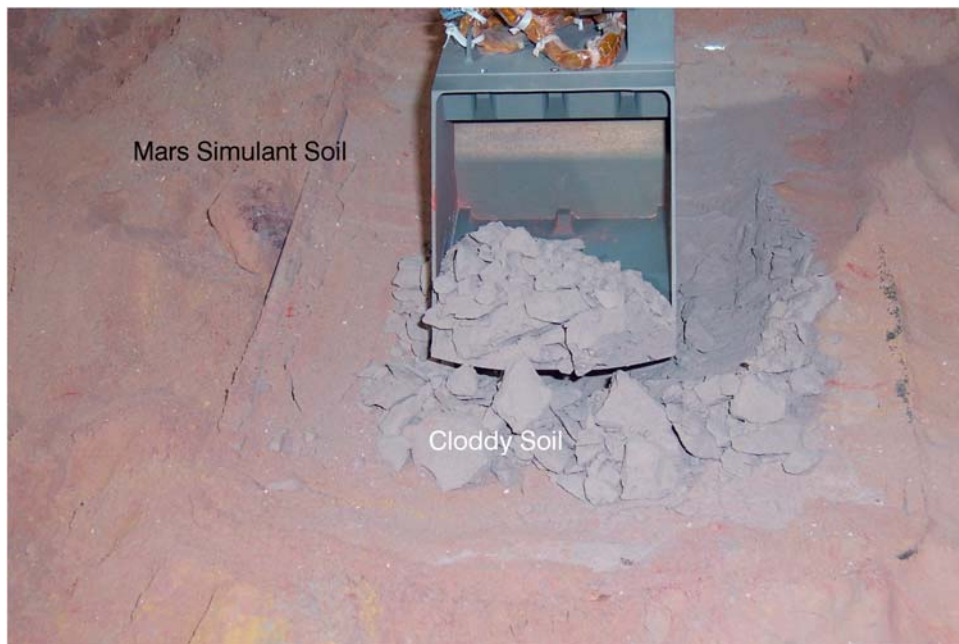
Figure 17. Laboratory excavation of a cloddy soil deposit using a flight-like RA and ISAD is shown in this color image. The cloddy soil simulant was prepared by taking ground basaltic sandy silt, saturating with water, and baking for 2 days at 100°C. This simulated crusty cloddy soil was then covered by several centimeters of loose soil simulant and the RA/ISAD was commanded to dig a trench. Note the platy nature of the clods, similar in appearance to the cloddy materials excavated from the La Mancha trench.
