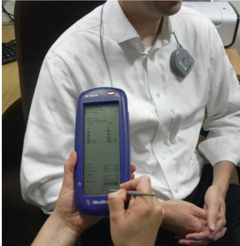
Figure 1.8: Titrating stimulation using a handheld programmer from Medtronic [28].
