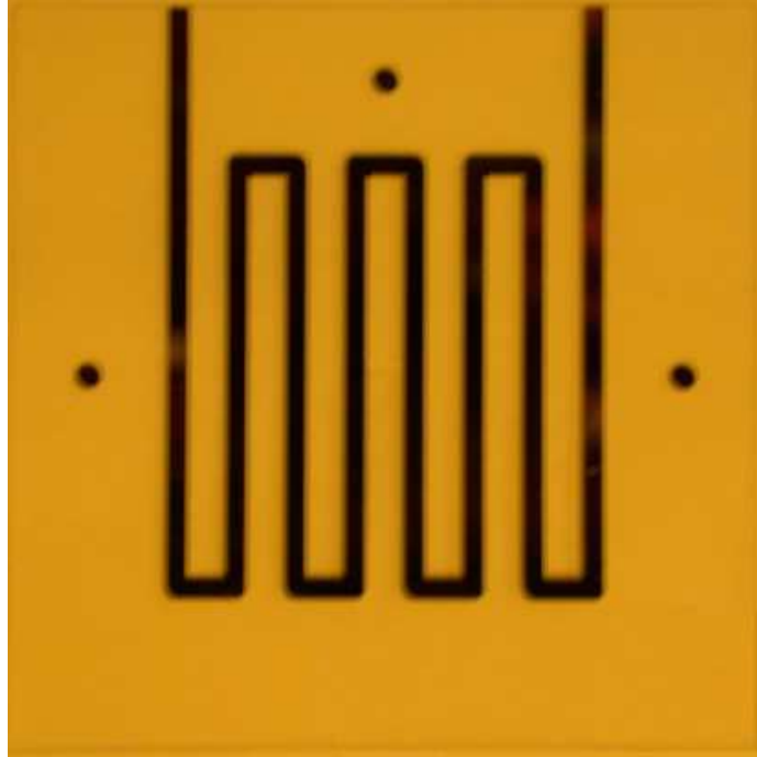
Figure 5.1: Platinum thin film heater deposited on a pyrex 7740 wafer
