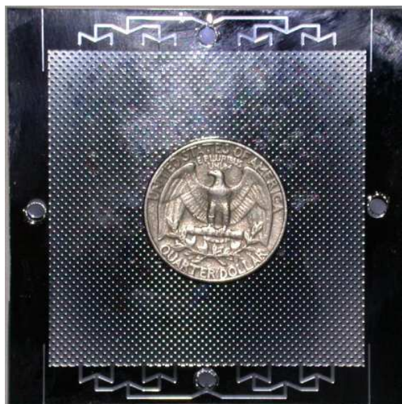
Figure 4.1: Silicon substrate based Preferential Oxidation(PrOx) micro-reactor
