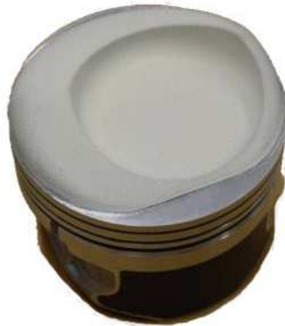
Figure 6.1 – Piston coated with 100 \mu m MgZr and an intermediate nickel alloy layer for stress relief
