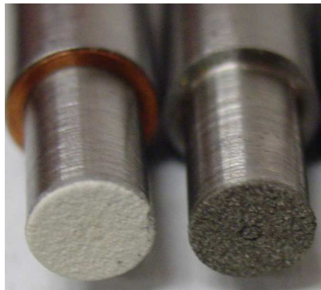
Figure 5.1 – Heat flux probes coated with MgZr with a nickel sub-layer (left) and the nickel layer alone (right)
