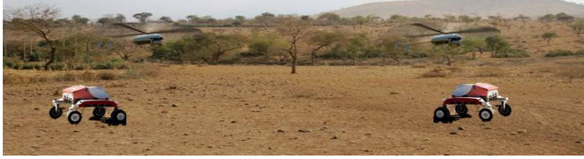
Figure 4.1: Transceivers and geolocation systems are mounted on robotic rovers or flyers that move in specified routes and acquire data about the subsurface environment (Image background borrowed from [6]).
