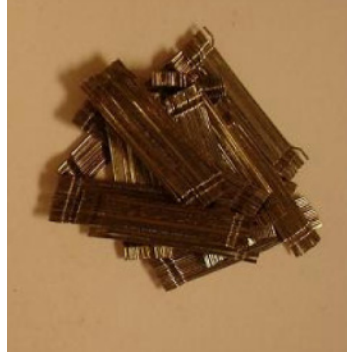
Figure 3.11 Dramix RC80/30 BP hooked steel fibers used in this study
