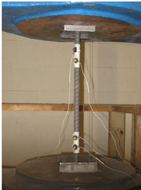
Figure 3.20 Direct tension test of a reinforcing bar using Optotrak markers to measure axial elongation
