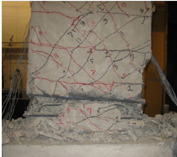
Figure 4.20 Damage in Specimen CB-4 at the bottom end of the beam at 3.7 % drift
