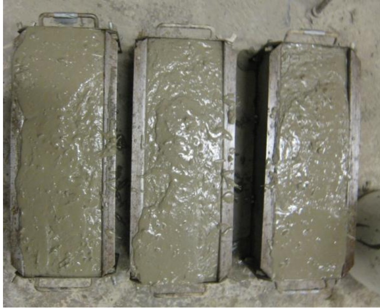
Figure 3.21 Casting HPFRC beams for flexural tests
