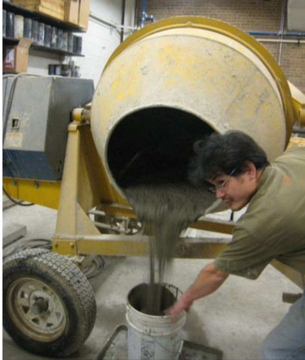
Figure 3.12 HPFRC mixture ready for casting
