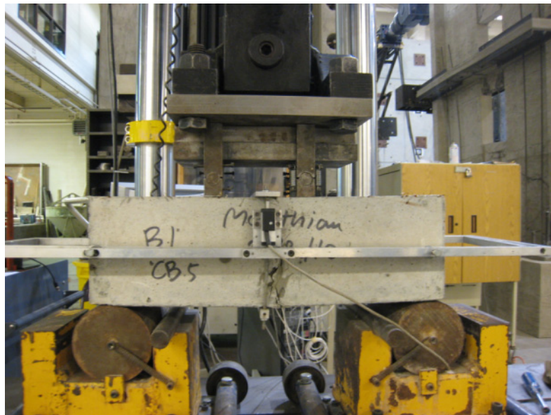
Figure 3.22 Test of HPFRC beam according to ASTM 1609-05
