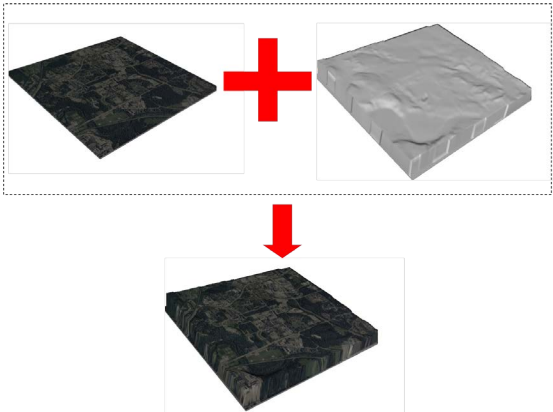
Fig. 2.14: Creation of 3D terrain polygon model using elevation data and georeferenced imagery
