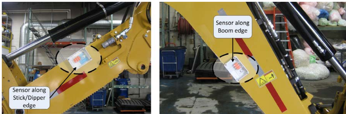
Fig. 5.7: Orientation sensors placed along the upper edge of the stick/dipper (left) and lower edge of the boom (right)
