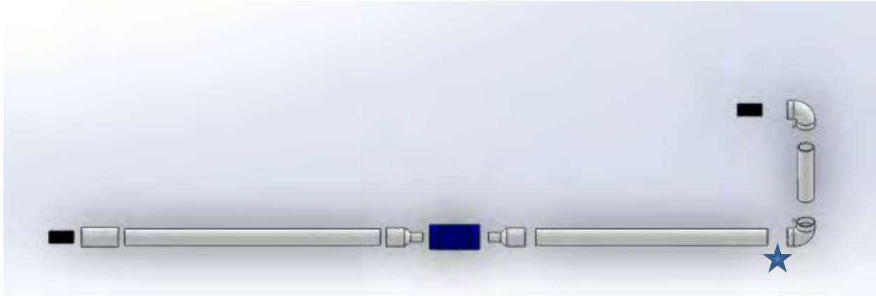
Figure 37. Exploded Side Pipe assembly. The starred joint should be dry fit and positioned before it is socket welded.
