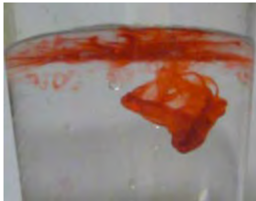
Figure 46. Diffusion process of the water soluble dye used in the dye tests, showing the somewhat chaotic diffusion process most likely do to Brownian motion
