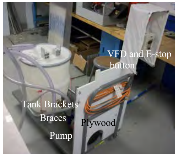
Figure 33. Cart containing tank, pump, and controls circuitry.
