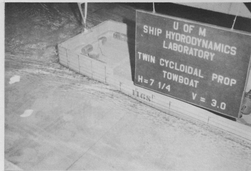
FIGURE 21 MODEL 1168 RESISTANCE TESTS AT VARIOUS WATER DEPTHS AT OR NEAR THE MAXIMUM SPEED FOR EACH DEPTH.
