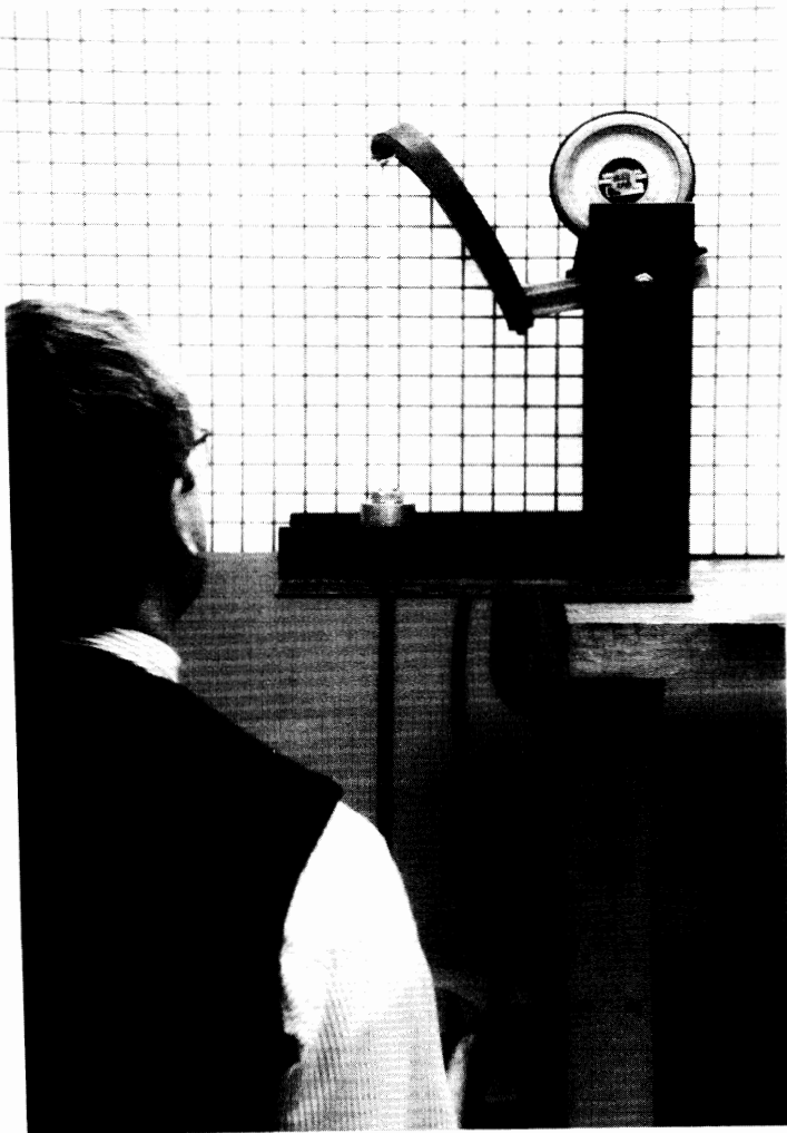
FIGURE 3-28a. Rib at initial angle of 10 degrees loaded with 6.8-kg (15-lb) mass in vertical direction.
