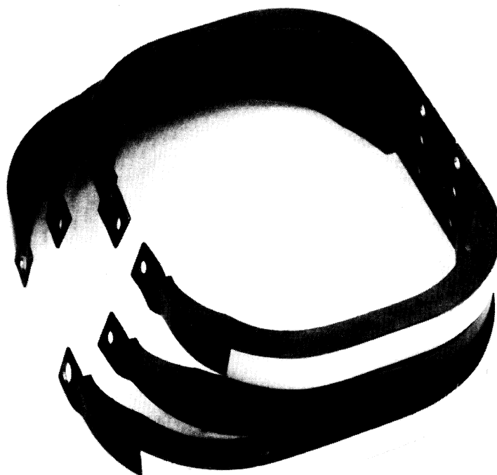
FIGURE 5-8. Top three ribs showing twisted tips for attachment of bib.
