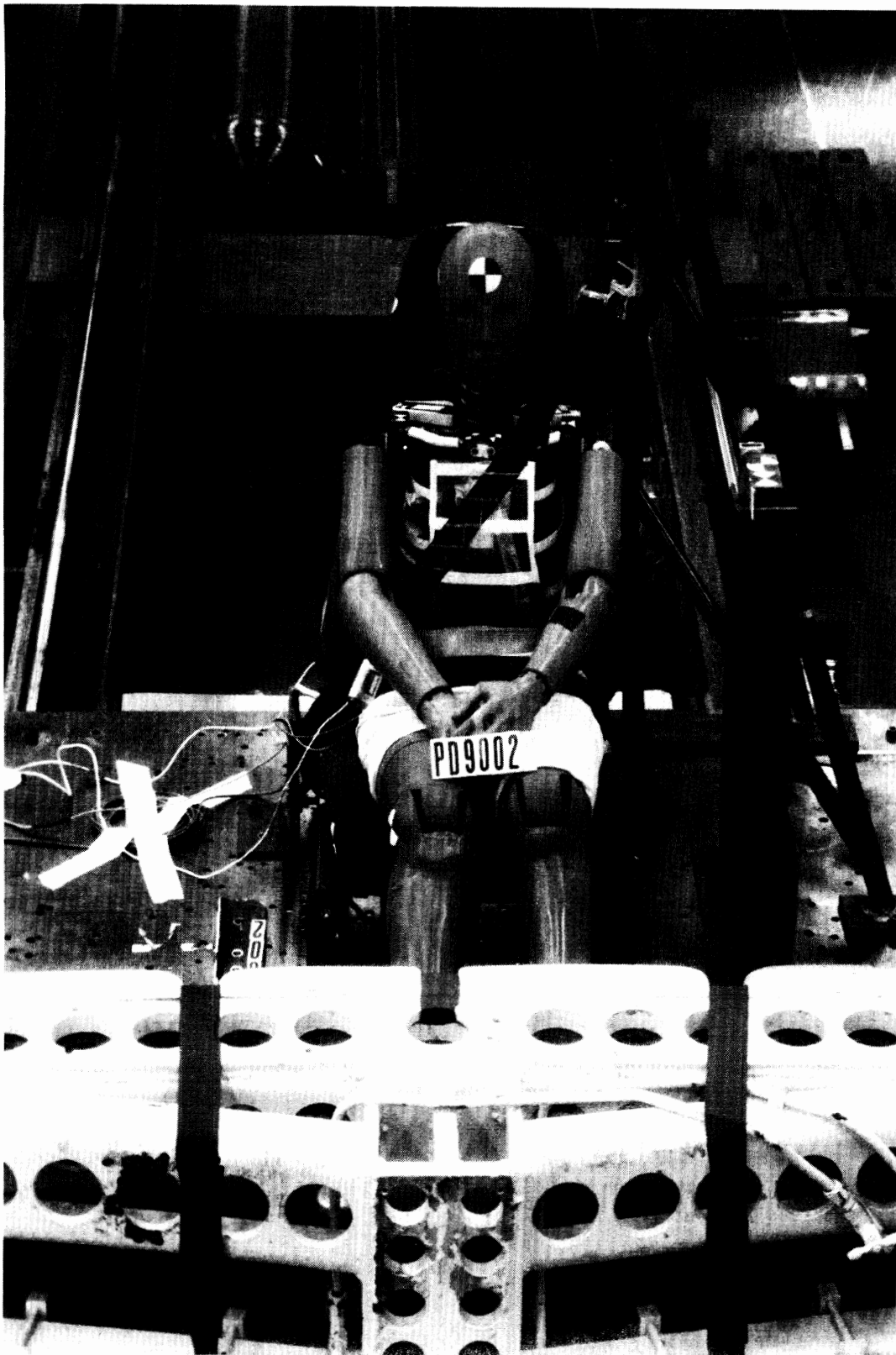
FIGURE 6-19d. Front view of sled test setup of First Prototype-50M dummy with more rearward position of right lap-belt anchor point.
