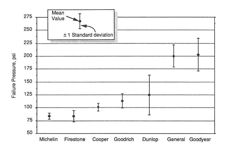
Figure 3. Failure Pressures by Tire Make
