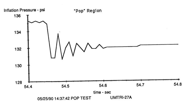
Dunlop A/P Radial Rover LT215/85 Rib Peak Pressure = 159.92 psi Popped Pressure = 138.64 psi Test ID 20
