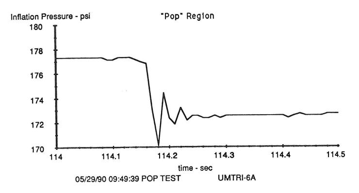
GoodYear Wrangler LT LT215/85 Rib Peak Pressure = 226.1 psi Popped Pressure = 168.26 psi Test ID 31
