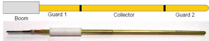
Figure 3. Langmuir probe designed at Penn State and used to measure the plasma characteristics in our test facility.
