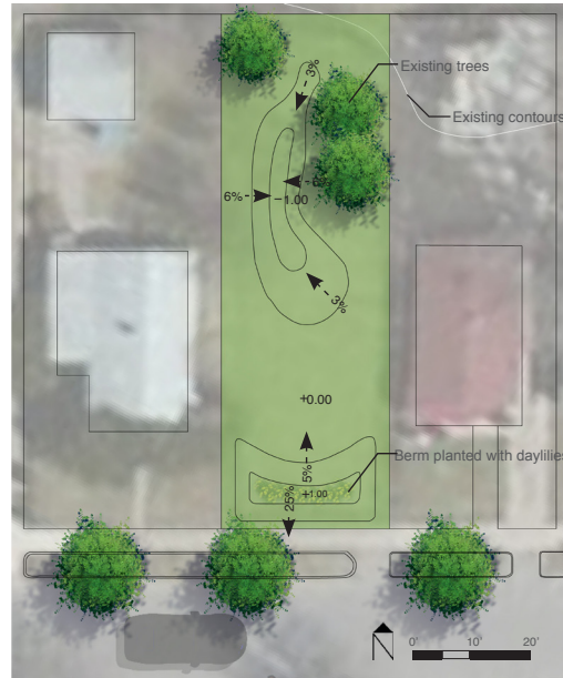
Figure III-1. Bioretention garden grading plan. Where trees are present on site, grading is completed outside of the dripline of existing trees. Perennials are planted on the low berm adjacent to the sidewalk.
