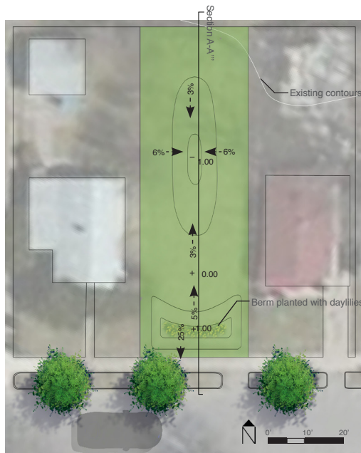
Figure III-1. Bioretention garden grading plan. Where trees are present on site, grading is completed outside of the dripline of existing trees. Perennials are planted on the low berm adjacent to the sidewalk.
