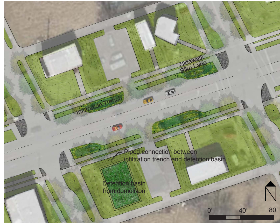
Figure V-11. Detail plan of connection between infiltration catch basins and infiltration garden from building demolition.
