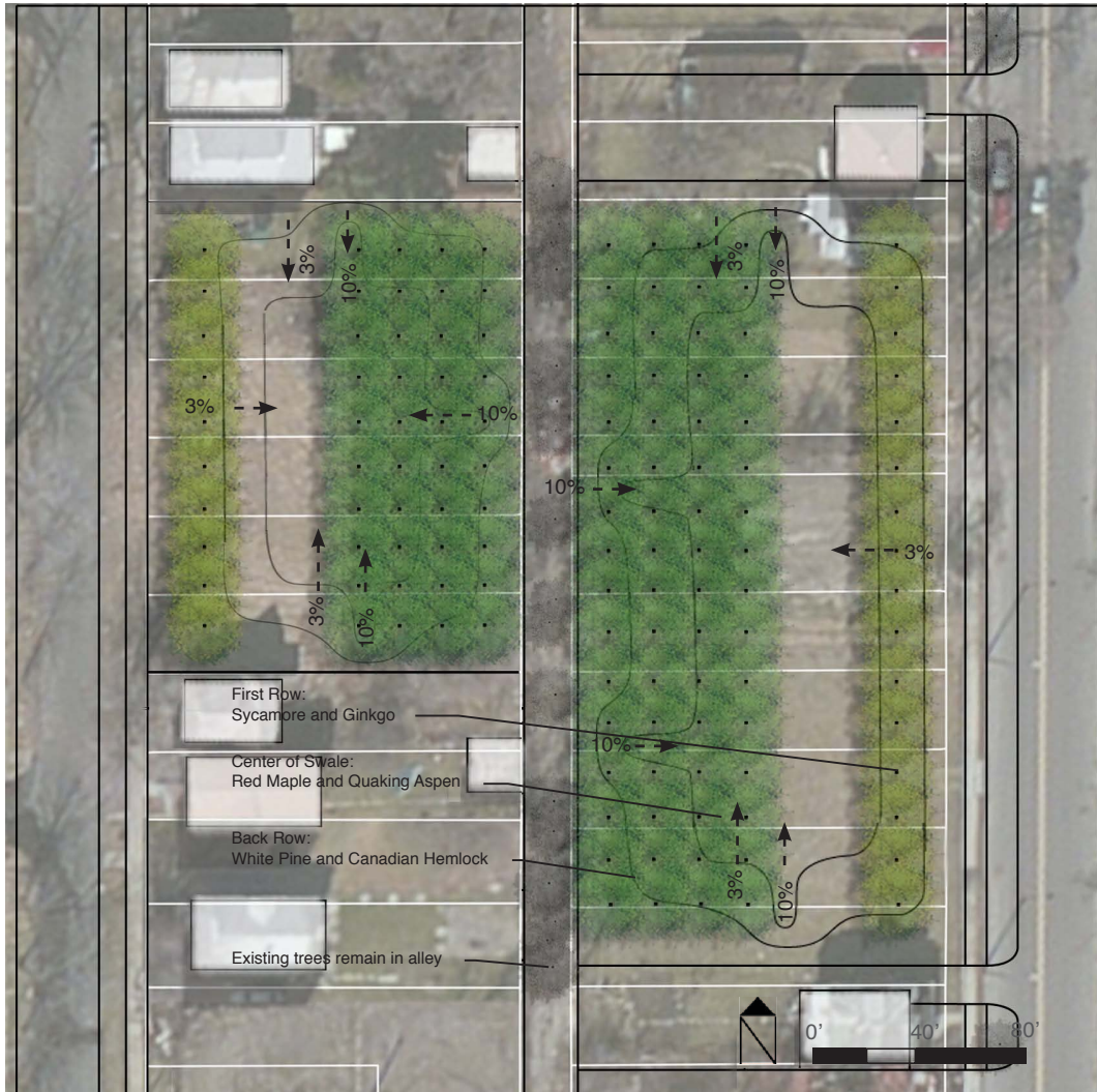
Figure III-23. Contiguous parcels within a medium urban woodlot may be located on either side of an alley. Existing trees remain in the alley.
