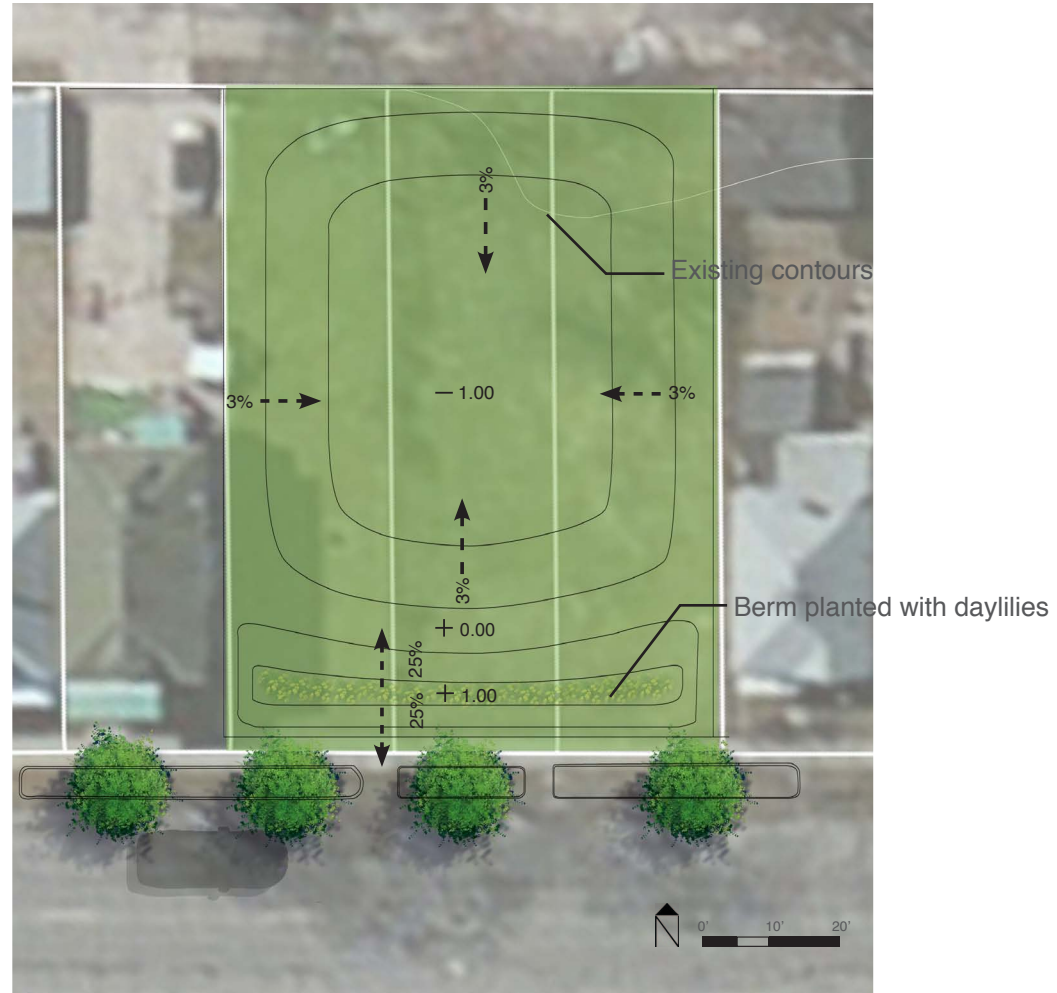
Figure III-5: Bioretention garden grading over three adjacent lots.
