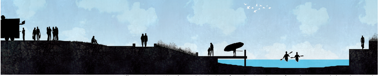
Illustration 31: Warehouse District Riverfront Section. Ramps from the proposed plaza down to the river create an accessible boat launch and an opportunity to directly access the river.
