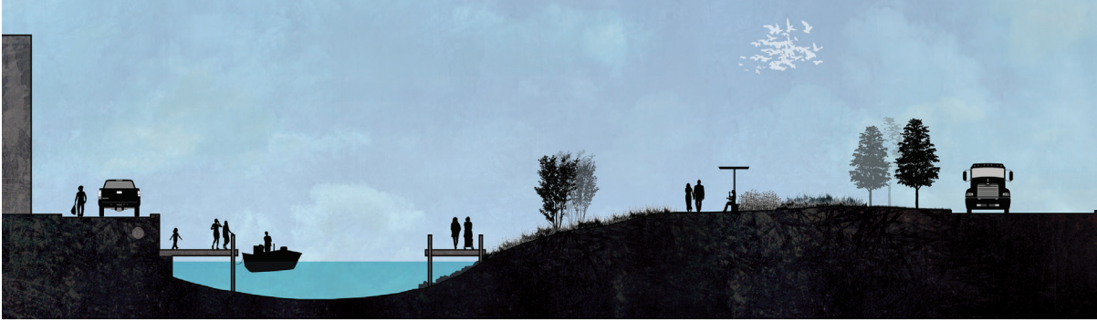
Illustration 19: 200 Block River Section. While vehicle access still dominates the south side of the Boardman, river access is introduced, giving boaters a place to tie up and visit Front Street. The banks on the right side boast a natural edge, and the 10' wide riverwalk allows access for a variety of users, while vegetation dampens vehicle noise from Grandview and creates a welcoming space.
