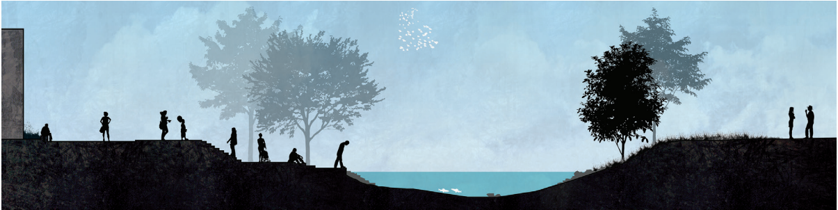
Illustration 21: Terraces River Section. Breaking down the retaining wall on the south side of the river allows for physical and visual access to the river in the heart of downtown Traverse City.
