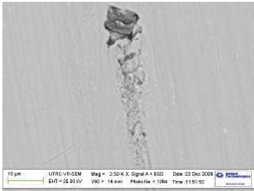
Figure 1.8 Carbide cracking after turning Inconel 718 (250×) [19]
