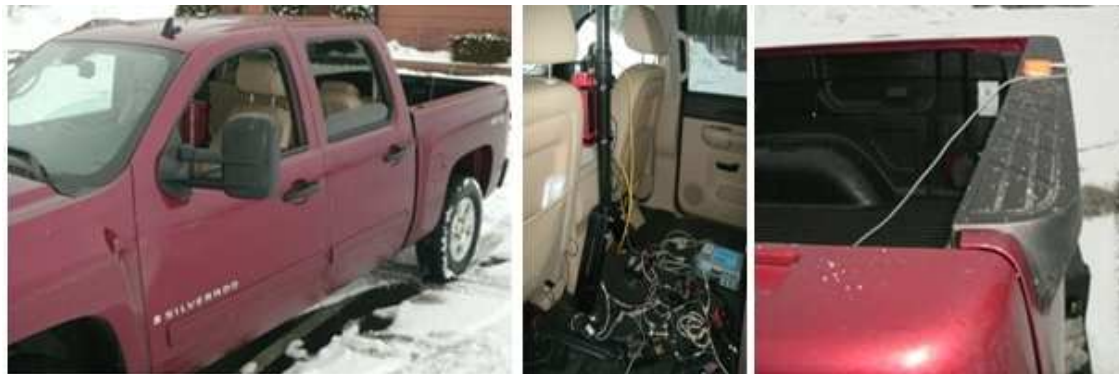
Figure 5.19 The test vehicle (GM Silverado) with equipment. (Left) The GPS receivers is located on the roof of the vehicle, (Center) The Oxford RT2500 is installed in the vehicle, (Right) The magnetometer is installed on the rear of the vehicle.
