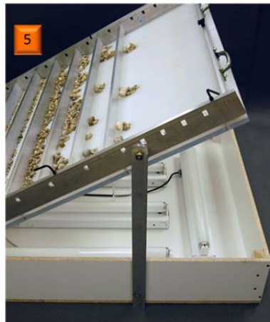
Figure 4.8 Immobilizing the inclined table
