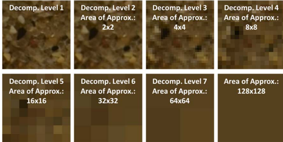
Figure 3.20 Seven levels of downscaling beginning with a 128 \times 128 image at PPD = 13.2
