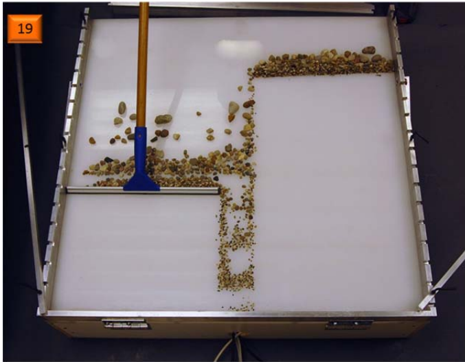
Figure 4.13 Specimen removal and cleaning
