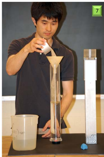
7 Pouring soil through funnel into the pre-segregation tube about half pre-filled with water.
