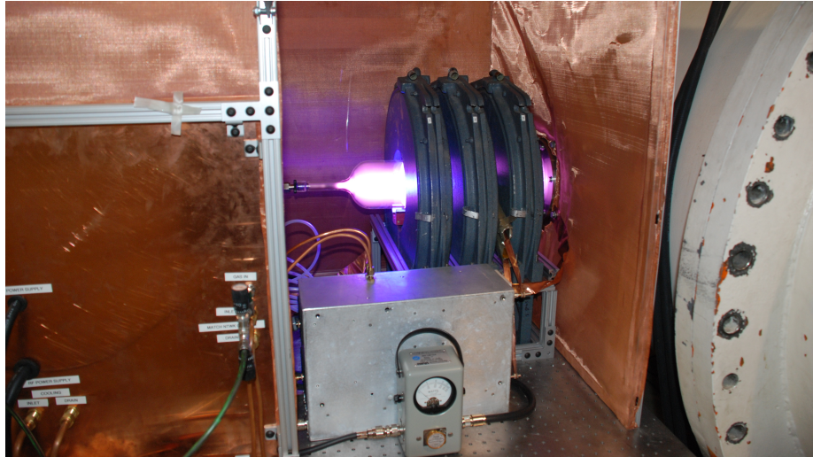
Figure 4.1: Setup of helicon plasma source for preliminary investigation.
