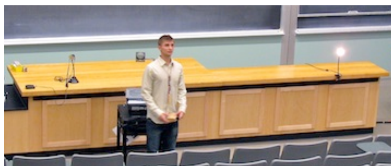
Fig 7a – The speaker is shown in the large lecture hall with three sources of IR light that can confuse an IR tracker.
