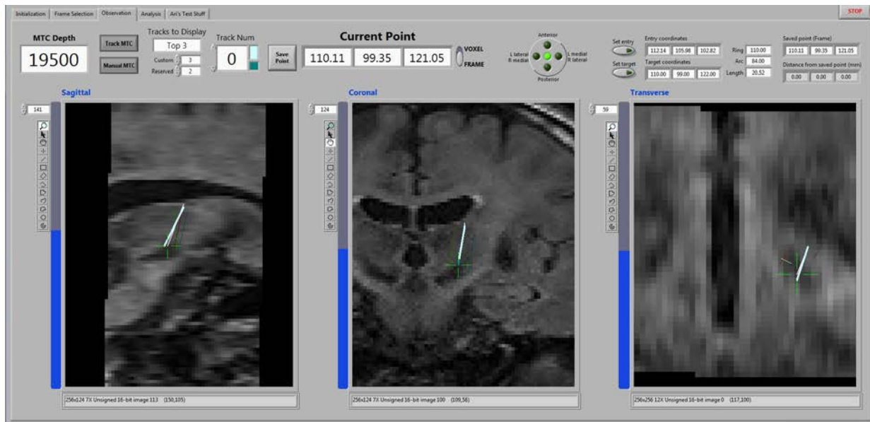
Figure 2.9: IODA’s alternate primary electrophysiological view. The display uses the patient’s preoperative MRI image and preoperative CT scan with frame to create an accurate frame-space image. The MER probe is superimposed onto the frame-based MRI image to show a real-time position of the probe as it traverses through the planned trajectory. Audio from the filtered signal is played throughout the trajectory.
