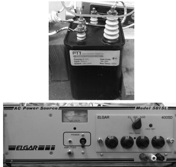
Figure 3.7: The Elgar A.C. power supply (bottom) and the high voltage transformer (top) used to drive bubble oscillations.
