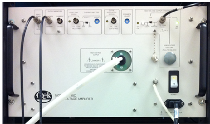
Figure 3.9: The TREK H.V. amplifier provides higher voltage and greater waveform control relative to the Elgar system. All input signals are provided by the Agilent arbitrary function generator.
