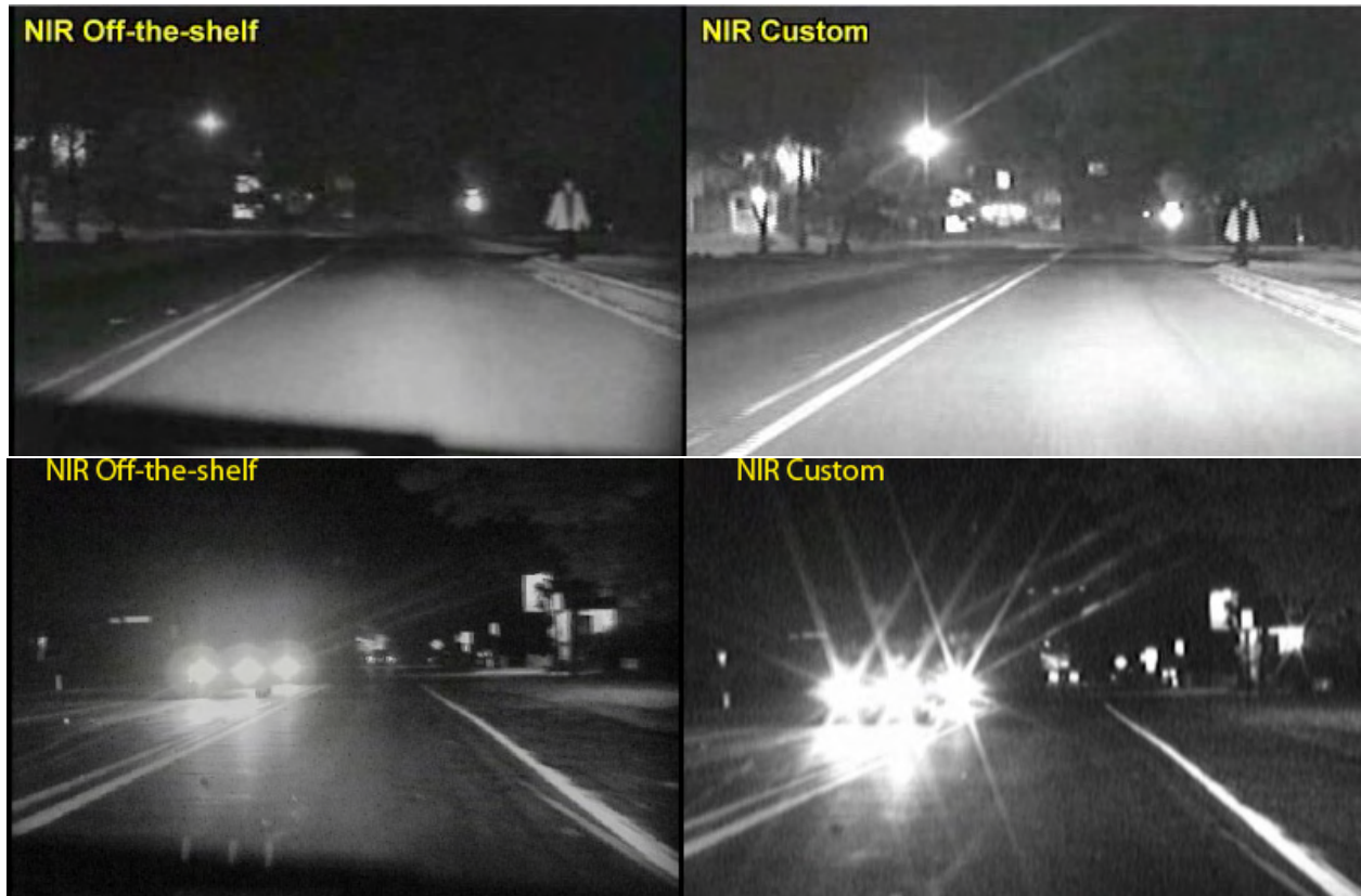
Figure 2. Visual comparison of image quality. Left: NIR off-the-shelf system; Right: NIR custom system similar to NIR from experiment.
