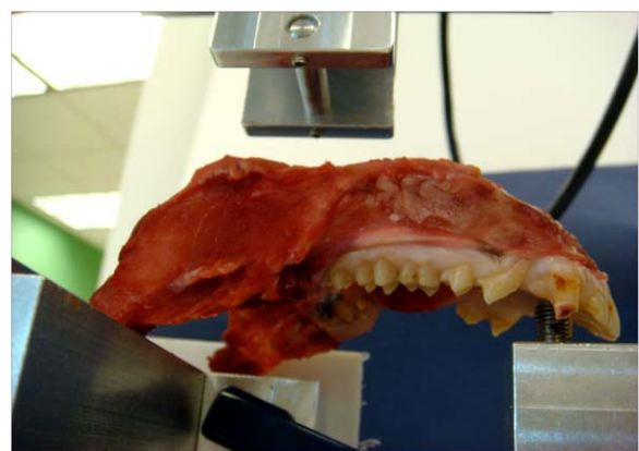
FIGURE 4. Each of the mandibles was placed on the three-point bending jig for biomechanical testing with the Alliance RT/30 Elite™ Controller. The jig model was designed by the Department of Biomedical Engineering, University of Michigan, Ann Arbor. The mechanical testing system was exposed to compression loads that simulated masticatory loads on each side of the mandible (reconstructed and non-reconstructed sides). Vertical linear displacement was applied by the Alliance RT/30 Elite™ Controller machine. [Color figure can be viewed in the online issue, which is available at wileyonlinelibrary.com .]
