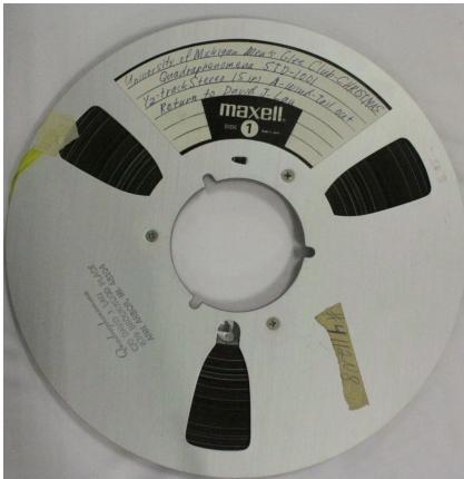
Left: A NAB Reel for professional recording; Right: Plastic reel used by both professional and amateurs
