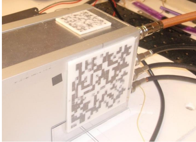
Figure 5.17: A 21 \times 21 random mask random mask pattern placed on the non-cathode side of a single detector.
