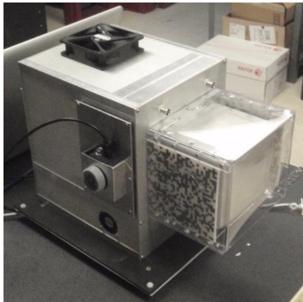
Figure 8.1: Polaris II system with two 32 \times 32 random masks applied to each 3 \times 3 array of detectors.
