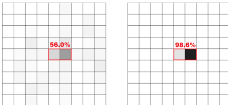
Figure 5.5 Repeatability of correctly identifying the Co-57 source direction using 500 measurements with 100 counts per measurement (left) compared to 500 counts per measurement (right)
